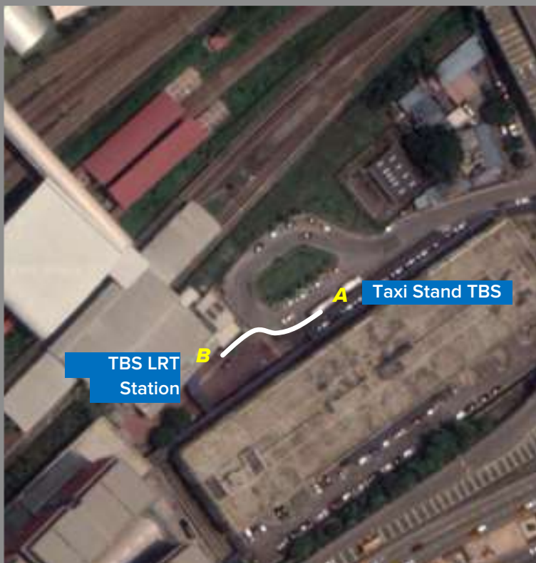
Fig. 23: Alignment of Proposed Improving Existing Walkway From TBS LRT Station to Taxi Stand TBS
