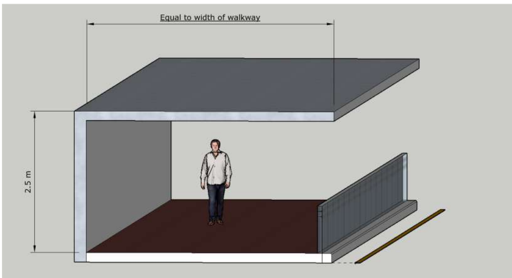
Figure 4.7 Schematic diagram of safety cover over walkway/bicycle lane
